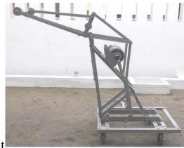
Winch arrangement (gauging Reel) with handle is fitted on the Crane. The current meter or Sediment Sampler is lowered or lifted by gauging reel easily. The gauging reel has capability to hold the current
