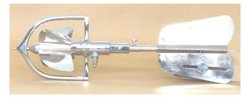
This "Instrumex" make Propeller Type Water Current Meter is used to measure Velocity of water flow directly in m/s. The spindle carrying the propeller wheel freely rotates in the pivot assembly. The magnet and reed switch assembly produces one pulse per rotation. The rotation of the Water Current Meter is sensed by sensor & gives pulsed output signal.
