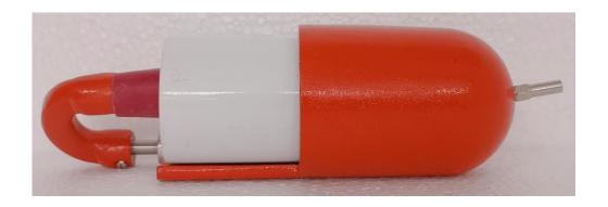
This is a lightweight sampler for collection of suspended-sediment samples where wading rod sampler suspension is used. The sampler consists of a streamlined aluminum casting, 13 inches (33 cm) long, which partially encloses a pint (0.47 liter) sample container (sold separately). The sampler weights 4.5 pounds (2 kg) including sample container. A standard 1/2 inch (1.27 cm) wading rod is threaded into the top of the sampler body for suspending the sampler.
