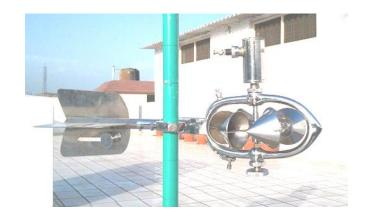
"Instrument" make Vertical Axis-Cup Type Water Current Meter is used to measure Velocity of water flow directly in m/s. The spindle carrying the cup wheel freely rotates in the pivot assembly. The magnet and reed switch assembly produces one pulse per rotation. The rotation of the Water Current Meter is sensed by sensor & gives pulsed output signal.
