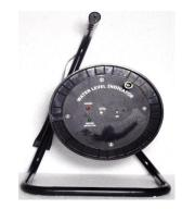
When the probe is touching the water-level there is a conductive connection between the tip of the probe and the sensor-body. Thereby a circuit of the lamp and the buzzer will be closed.
