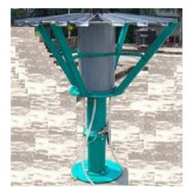
snow collection by blowing the snowfall away from the funnel/collector. The design of the Alter style wind screen prevents strong updrafts and induces turbulence around the snow gauge funnel / collector. These actions aid to reduce air flow streams over the snow gauge funnel / collector and result in better collection of the snowfall during windy conditions. Significant increases in the gauge catch are noted whenever the snowfall size is very small.
